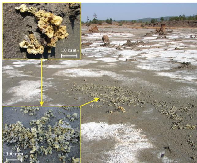
Fig. 1. Efflorescent minerals on the surface of a Karabash mine tailings – postmining minerals that form due to evaporation, as surface encrustations.
