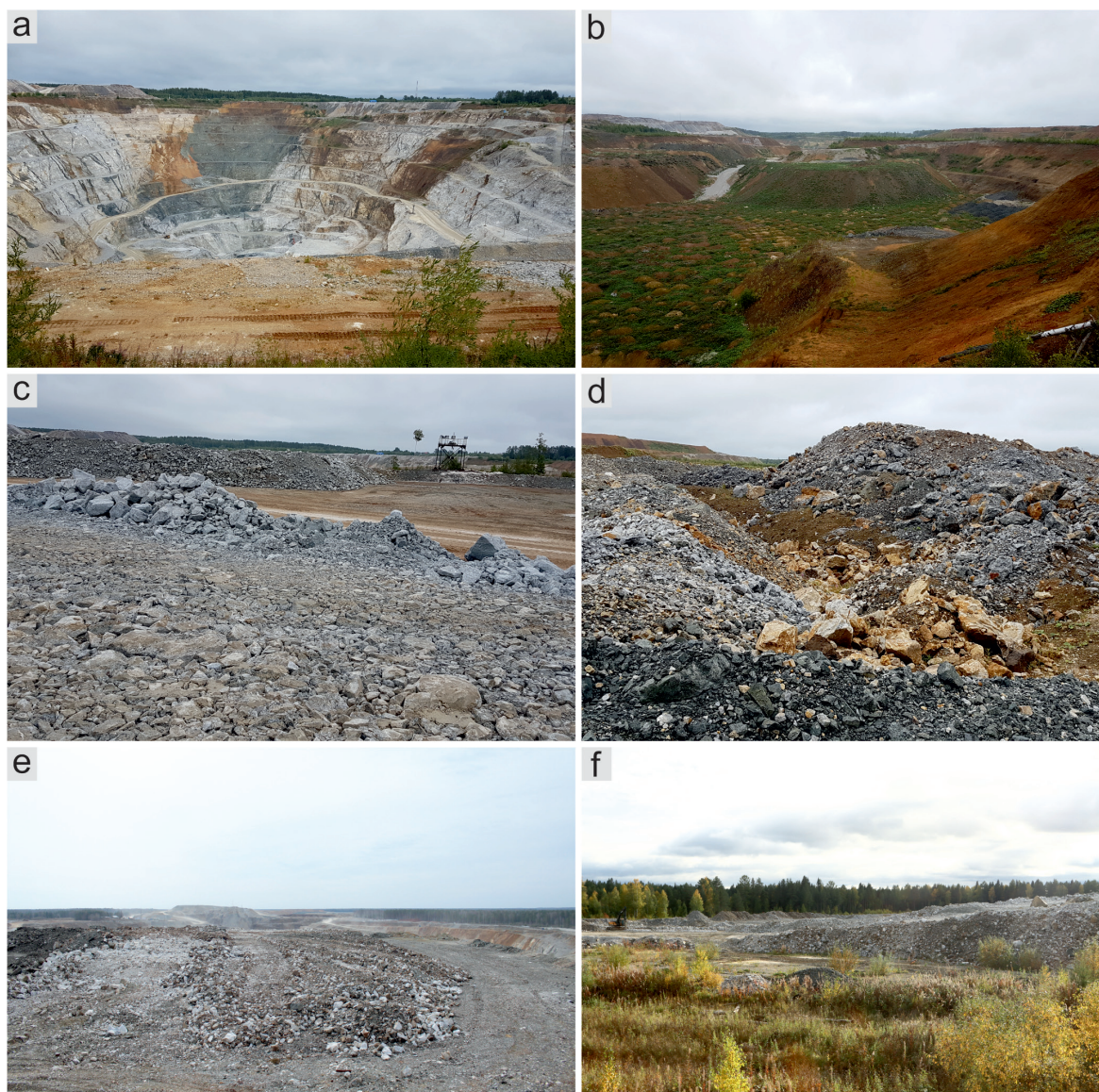
Fig. 2. Main sites of the mine operating at the Vorontsovskoe deposit: a – northern open pit; b – southern open pit; c – main ore stockpile; d – dumps of northern open pit; e – off-balance ore stockpile no. 1; f – off-balance ore stockpile no. 2.
