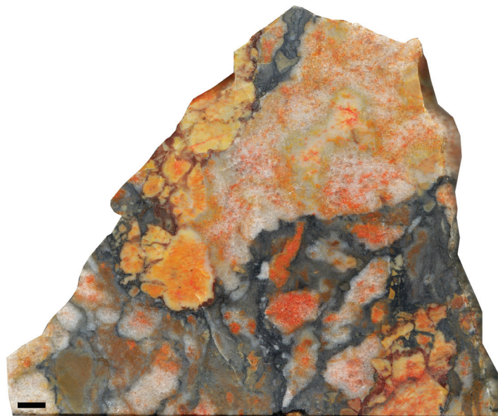
Carbonate breccia with As mineralization from the Vorontsovskoe deposit (sample of Elena Belogub, scale bar is 1 cm)
